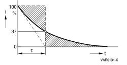
Figure 7 Time constant of flywheel circuit
