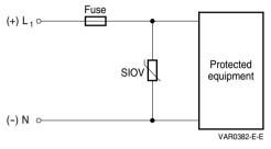
Figure 1 AC/DC single-phase protection
