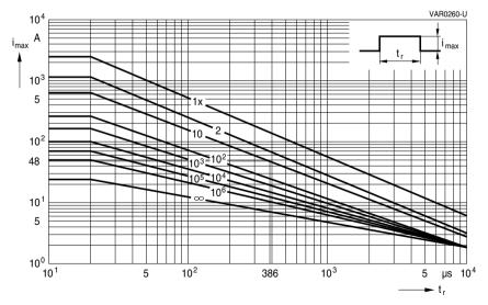
Figure 21 A maximum surge current  $i_{max}$  = 48 A (ten times) can be deduced for  $t_r^*$  = 386 µs from the derating curves for S10K50 ... 320
