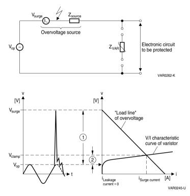
Figure 2 Principle of overvoltage protection by varistors
