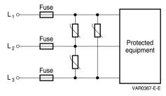
Figure 2 AC three-phase protection
