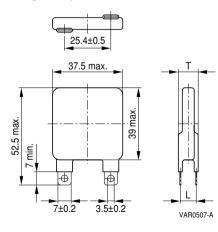
Ordering code T<sub>max</sub> L+1.0 mm mm B72240L0131K102 8.1 4.4 8.2 4.5 B72240L0141K102 B72240L0151K102 8.3 4.6 B72240L0231K102 9.0 5.4 B72240L0251K102 9.2 5.6 B72240L0271K102 9.4 5.8 6.3 B72240L0321K102 9.9 B72240L0381K102 10.6 6.9 10.9 7.3 B72240L0421K102 B72240L0441K102 11.1 7.6 B72240L0461K102 11.4 7.8 B72240L0551K102 12.3 8.8 B72240L0681K102 13.5 9.9 B72240L0751K102 14.1 10.5
