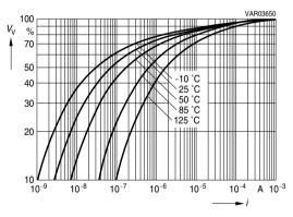
Figure 18 Typical temperature dependence of the V/I characteristic taking SIOV-S20K275 as an example.
