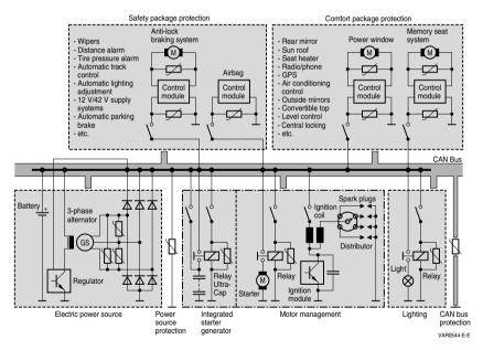
Figure 9 Automotive electrical system, complete EMC concept with varistors
