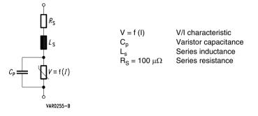
Figure 16 Varistor model, basic structure
