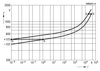
Figure 4 Tolerance band of the SIOV-B40K275
