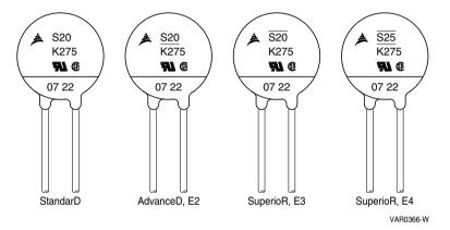
Figure 21 Various forms of printed markings of disk-type varistor series StandarD, AdvanceD and SuperioR, using S20K275 as an example. Date code 07 09 ≙ yy ww ≙ 9th week of year 2007
