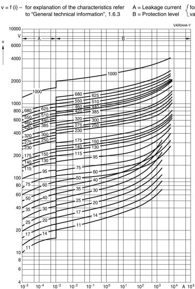
A = Leakage current ∫ for worst-case B = Protection level varistor tolerances
