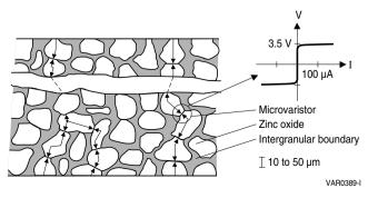
Figure 3 Conduction mechanism in a varistor element
