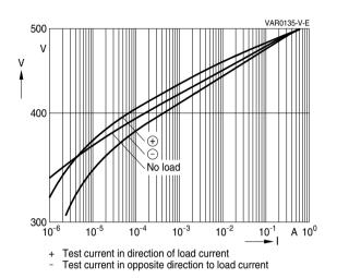
Figure 12 Typical polarization effects of leakage current for unipolar loading of metal oxide varistors
