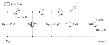
Figure 18 Simulation of the test pulse 10/700 µs applied to the device under test S10K95
