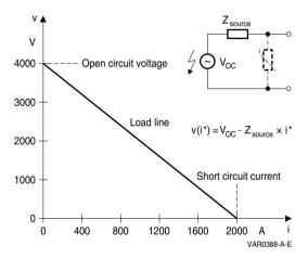
Figure 5 Load line on linear scale
